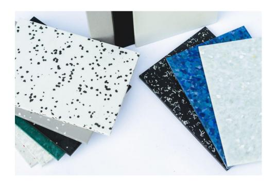
Being a truly circular product, Polygood® is composed of recycled refrigerator and freezer insulation, household electronics, CD disk cases, single-use cutlery, toys, games, cables, acoustic panels, and tubing. At the end of its useful life, the company offers a free Take-Back Programme that recycles old panels for future projects.
