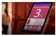
The Z+ People Counter works thanks for a camera tracking system which is incredibly easy to implement. The device accurately regulates the number of people going in and out of any entry/exit point of a building or enclosed area within a building. Non-emergency application is possible thanks to software which provides statistics on visitors so you can use them to optimize your business.
