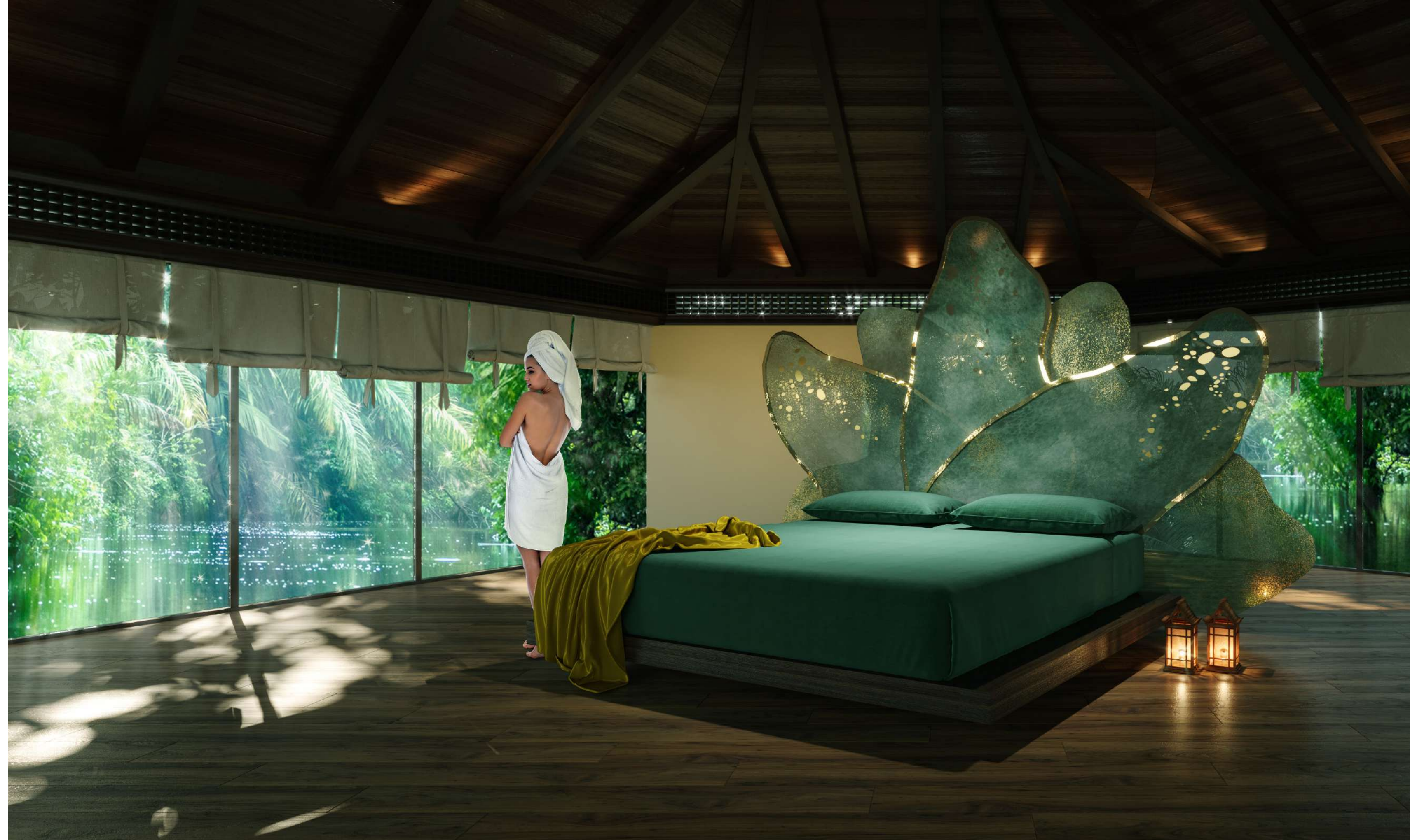
Headboard composed by seven extra-clear, shaped, melted glass sheets, thickness 10 mm. each, with sandblasting, gold coloured leaf inserts, "Trilli Effect" (golden powder), green/blue shades digital printed. Laser cut "U" shaped stainless steel frame covered with gold coloured leaf.
