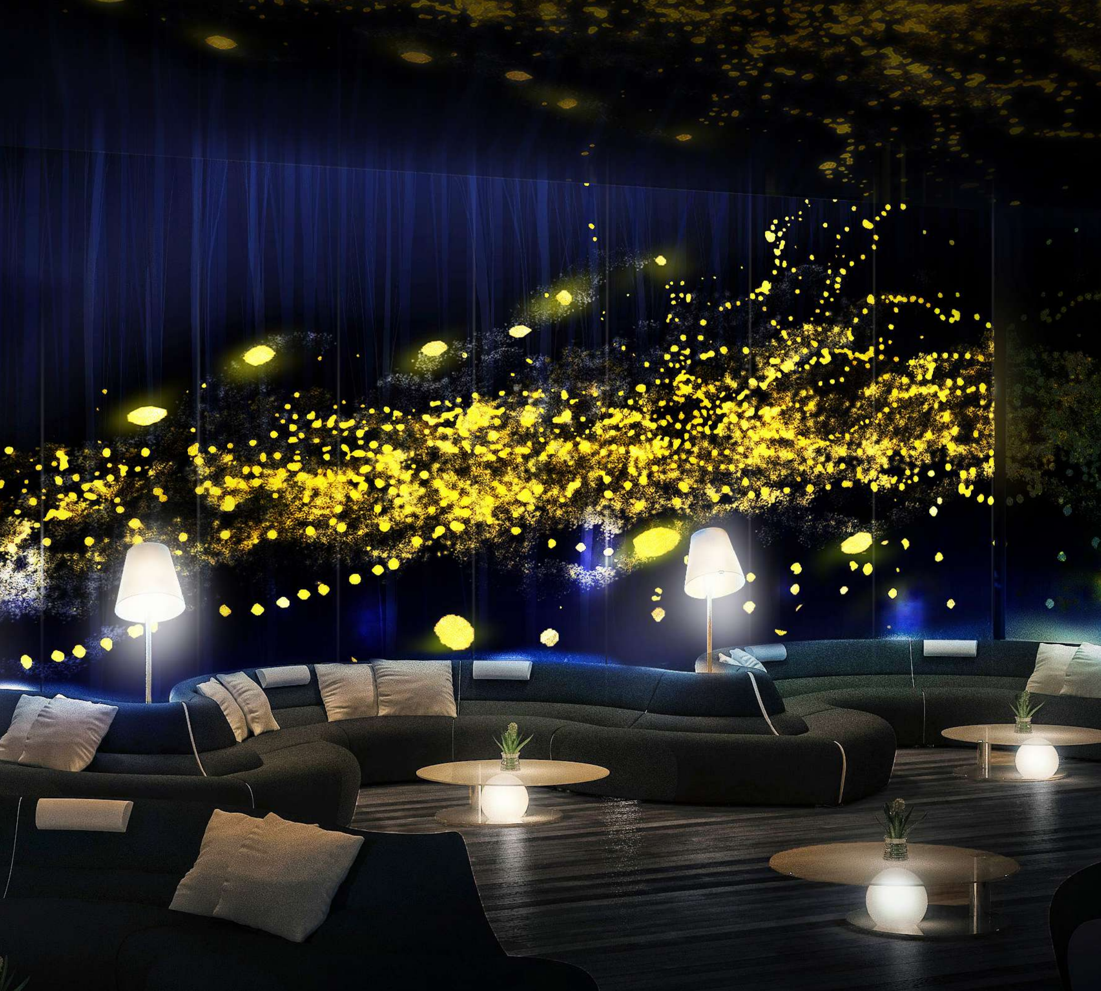
Single face extra-clear tempered glass wall 12 x 3,5 m., extra-clear, tempered, composed by 12 sheets 1 x 3,5 m., thickness 10 mm. decorated with digital printing, sandblasting, gold leaf application, and blue painting.
