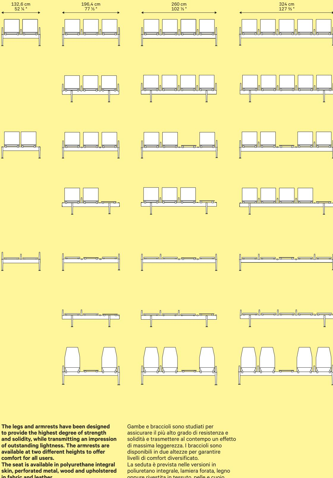
The legs and armrests have been designed to provide the highest degree of strength and solidity, while transmitting an impression of outstanding lightness. The armrests are available at two different heights to offer comfort for all users. The seat is available in polyurethane integral skin, perforated metal, wood and upholstered in fabric and leather.
