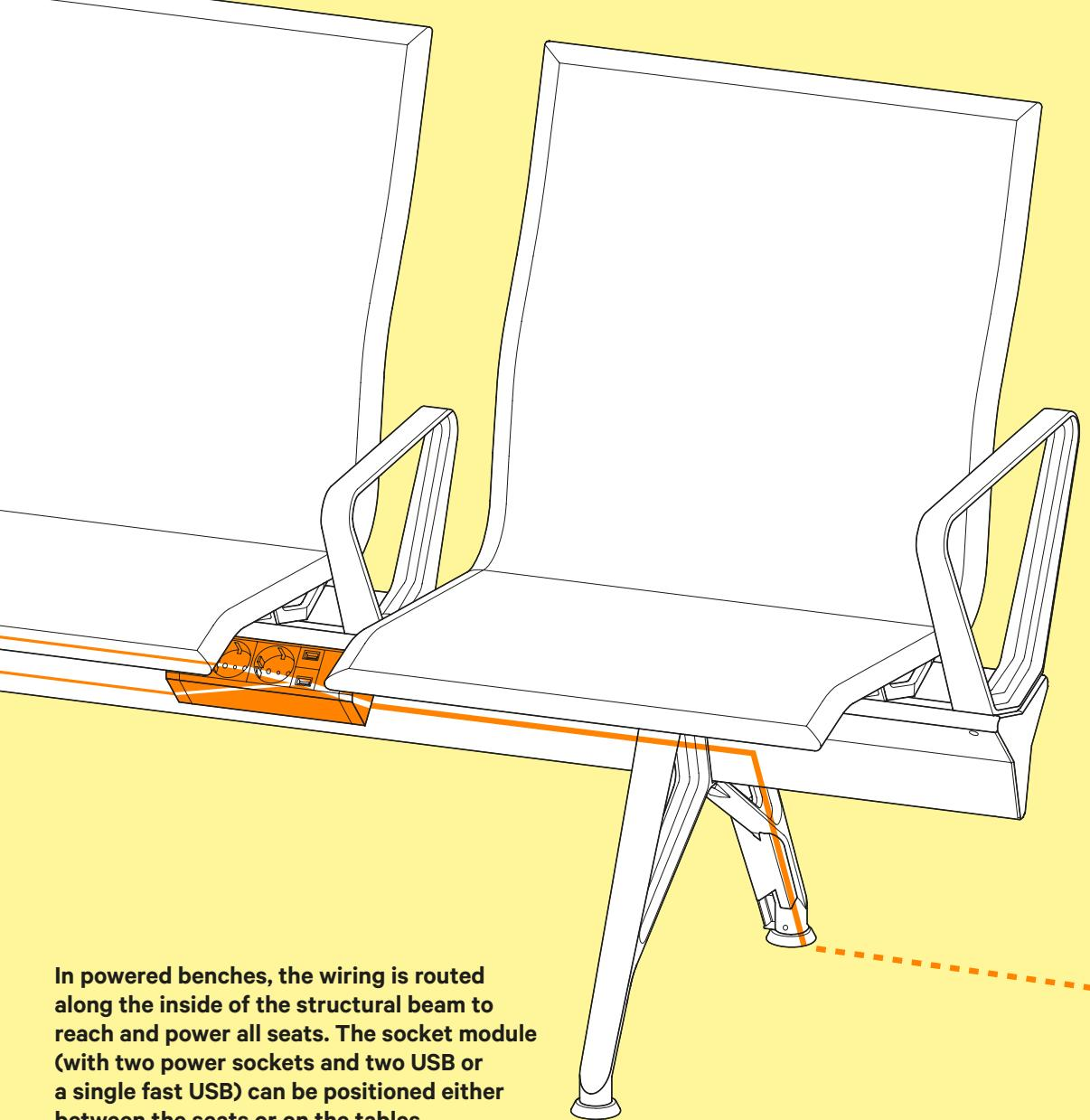
**In powered benches, the wiring is routed along the inside of the structural beam to reach and power all seats. The socket module (with two power sockets and two USB or a single fast USB) can be positioned either between the seats or on the tables.**
