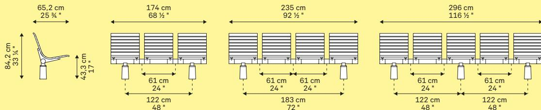
**Aluminium backrest seat with armrest direct floor fixing base**
