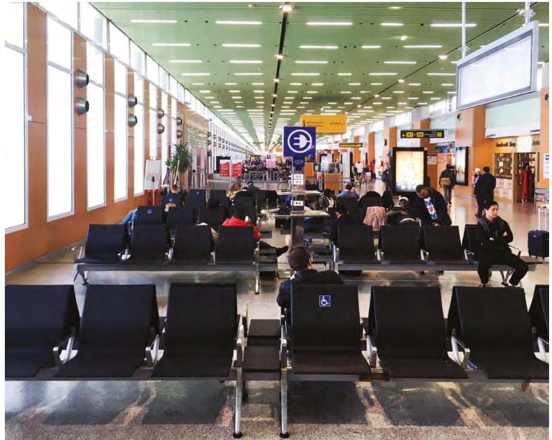
**The one-piece structure of the polyurethane seat makes the entire composition dynamic and streamlined: the ergonomic design features a double-S profile for lumbar support, while the rounded profile of the front of the seat allows unimpeded circulation in the legs. The design of the seat means it retains the body's natural posture even for long waiting times.**
